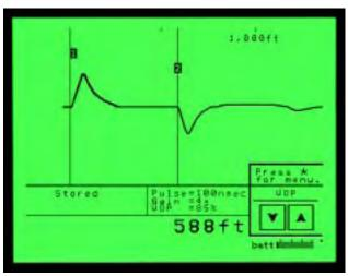
Selected functions and operations are controlled by the keypad, such as waveform position, horizontal zoom, vertical gain, cursors, range, contrast, and backlight. A popup menu is easily accessible for additional functions. Riser-Bond Instruments' unique popup menu system allows the operator to quickly select and use a function while the waveform is active.
